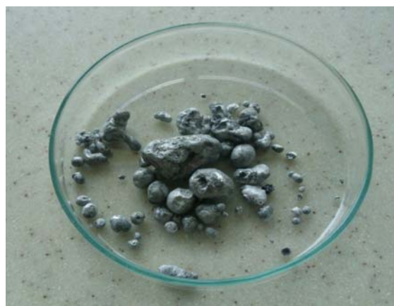
Fig. 5: Photo image of recovered aluminum from orange merinda can denoting visible holes and dendrites.
