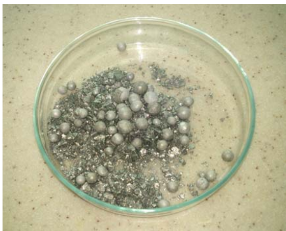
Fig. 6: Photo image of recovered aluminum from pepsi cola can showing smooth surfaces.
