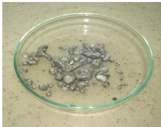
Fig. 4: Photo image of recovered aluminum from orange merinda can showing visible craters
