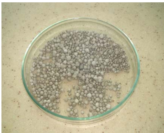
Fig. 7: Photo image of recovered aluminum from coca cola can showing smooth surfaces.
